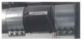
When highly charged edge trim passes through the ionization chamber seen above, the flood of free ions drenches and neutralizes the static charges.
